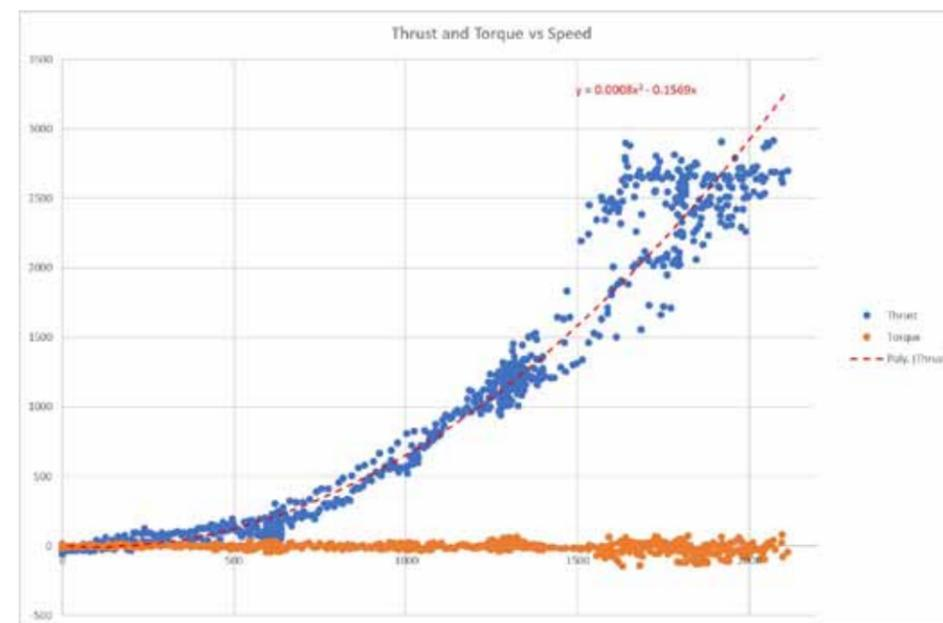
Combined motors - net torque close to zero
