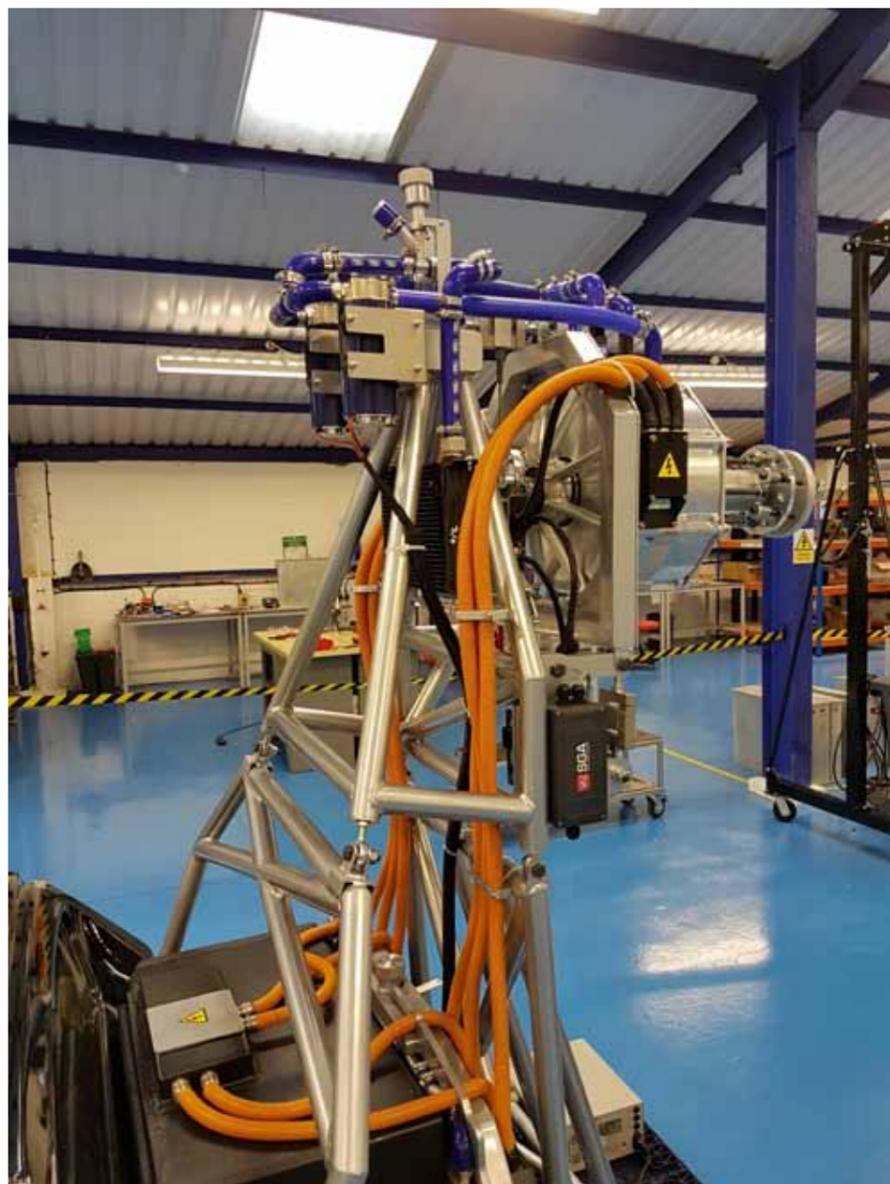
ABOVE: the CRPS fitted to the test frame complete with cooling system and instrumentation. The assembly weighs 88kg
