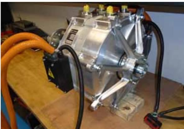
TOP TO BOTTOM: mechanical simplicity – the two splined collars (right in photo) bolt directly to the rotor inside each motor. The longer of the two shafts fits inside the short outer shaft, which has an integral propeller hub, to form the coaxial contra rotating assembly (the second propeller hub is not shown); CRPS drive unit, showing the front bearing support and coaxial shaft with twin propeller hubs; and a rear view of the same, showing the rear bearing support for the coaxial shaft assembly
